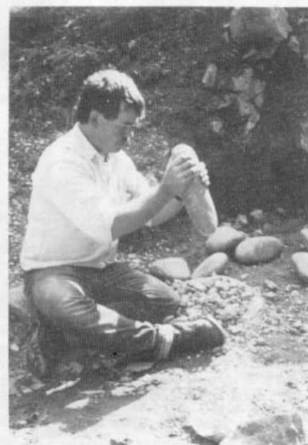
Plate 2. Ore-dressing with hammerstone.
